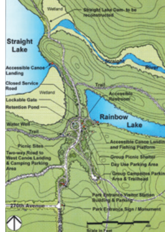
An example of a conceptual site plan. Proposed park development is shown in relation to the property's topography and natural features.
