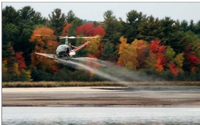
Pilot Rene "Sparky" Stimart of Skyline Helicopter used his small and highly maneuverable craft to spray a mixture of water and rotenone on Lake Tomah. The spray jets created large droplets so there was no misting and the mixture fell entirely on the lake.
