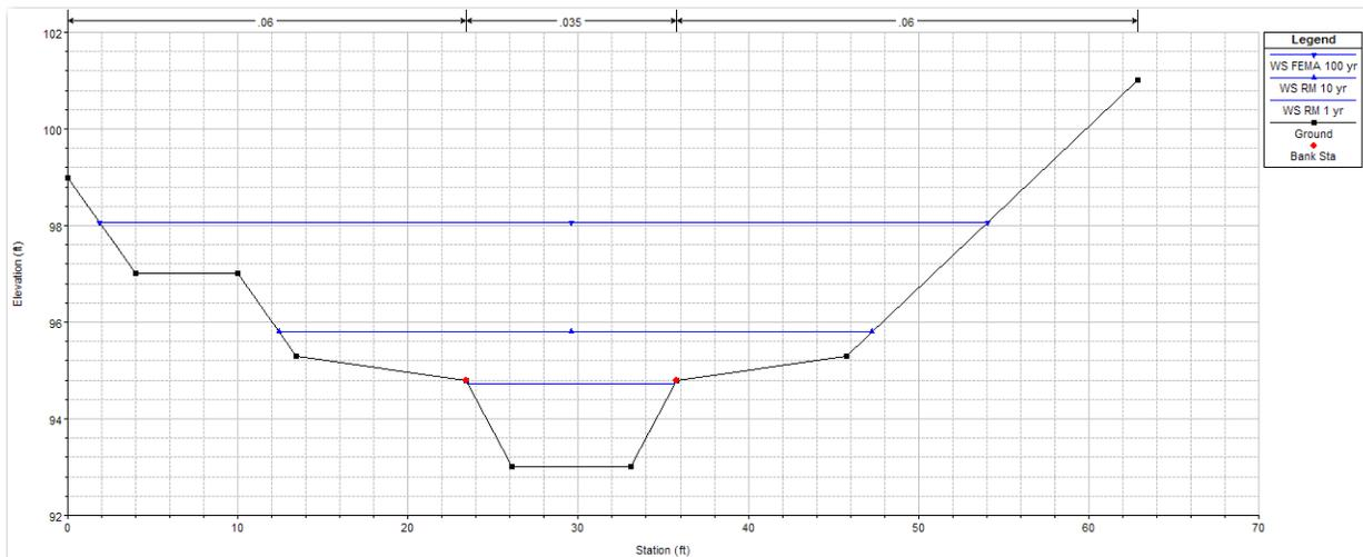
The predicted flood profile for the 100 yr flood event was compared to that in the FEMA Flood Insurance Study to ensure that flood elevations are not increased anywhere along the profile. As expected, the rehabilitated channel caused decreases in flood elevations by creating additional flood storage. Flood water that currently backs up upstream of the existing culvert and eventually covers the parking lot would be stored within the new stream valley below the parking lot elevation.
