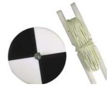
*Figure 3: A Secchi disc, which is lowered into the water to measure water clarity*
