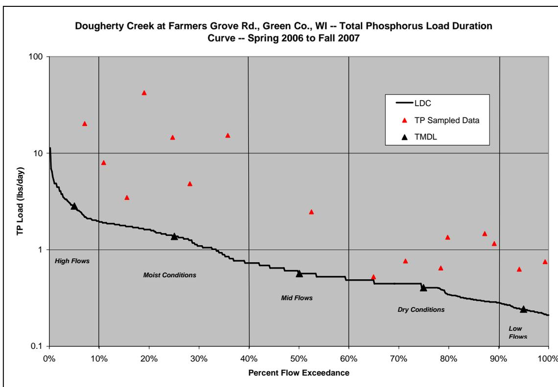
**Figure A-1.** Dougherty Creek Load Duration Curve for Phosphorus. This figure shows that all sampled total phosphorus data was above the target value under all flow conditions.
