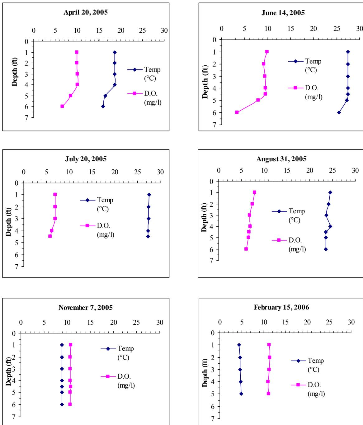
Figure 6. Williams Lake dissolved oxygen and temperature profiles collected during 2005 and 2006.
