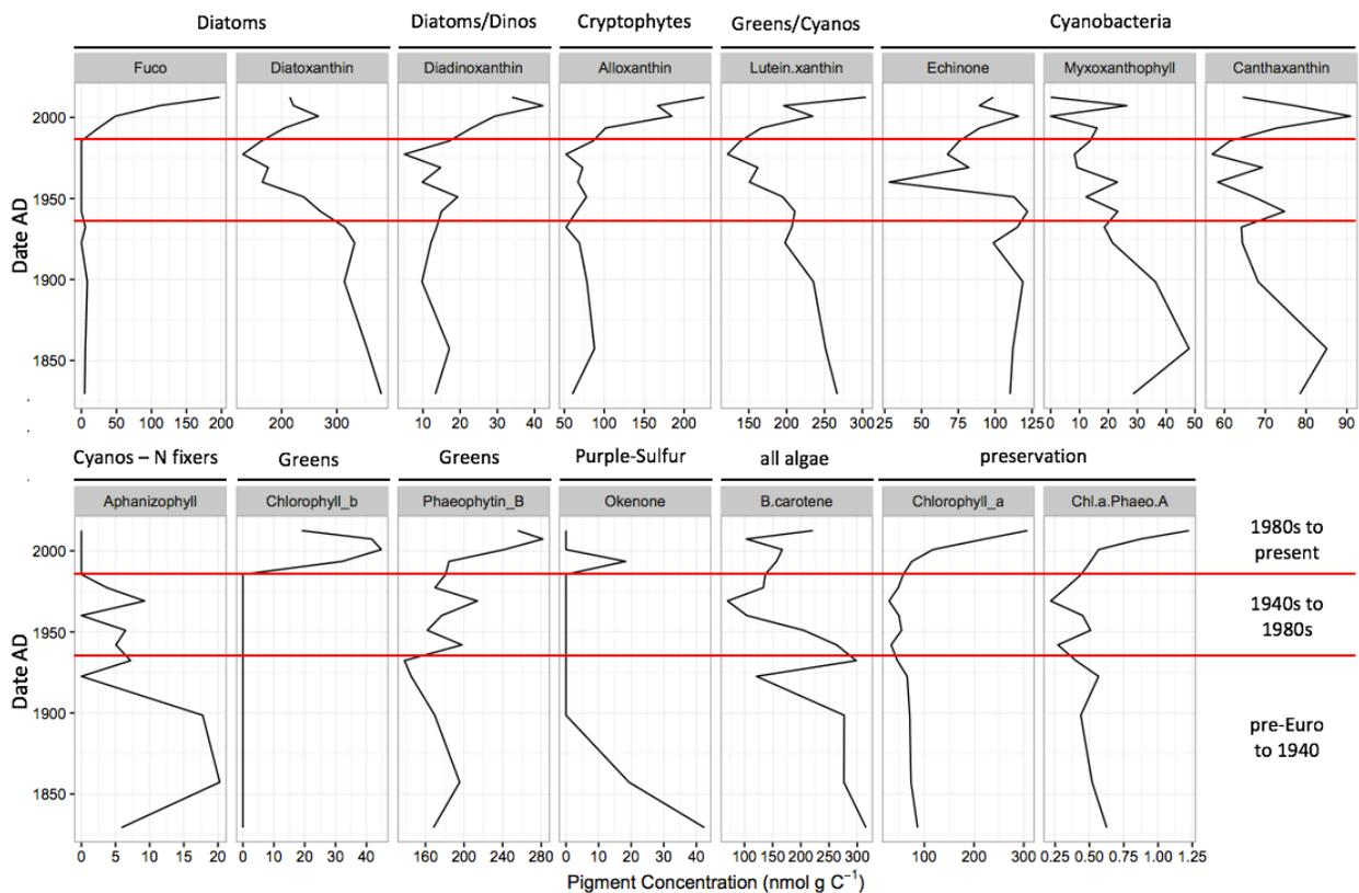
Fig. 1. Downcore profiles by date (AD) of fifteen photosynthetic pigments or indicators (nmol gC<sup>-1</sup>) in Bone Lake. Pigment source or indicator value noted above each graph. Red lines denote major periods of historical change in algal communities.
