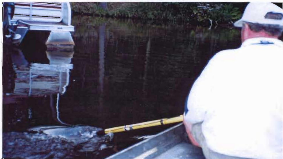
Figure 9. The submerged probe used in the conductivity survey is shown here. The entire nearshore area of Big bear Lake was surveyed.
