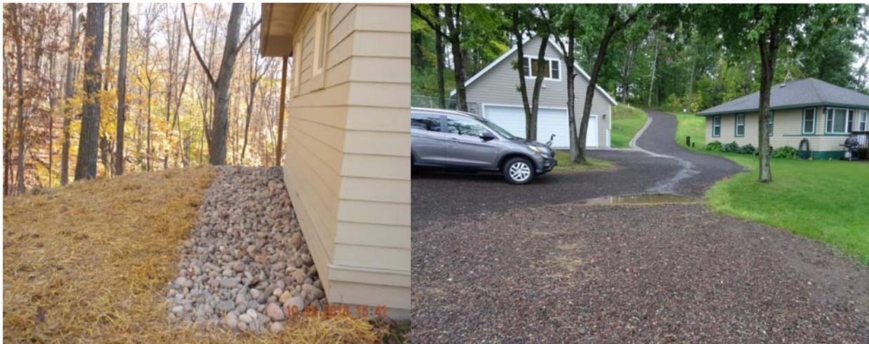
**\*Diversions** redirect runoff that would otherwise move downhill into the lake to an area where it can soak into the ground. Diversions may be used in connection with rock infiltration or rain gardens. Diversions include berms, trenches, and water bars.
