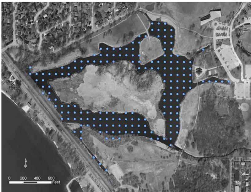
Figure 5: Point intercept sampling grid for Verona Quarry
