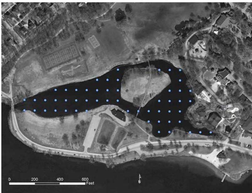
Figure 4: Point intercept sampling grid for Warner Park Lagoon
