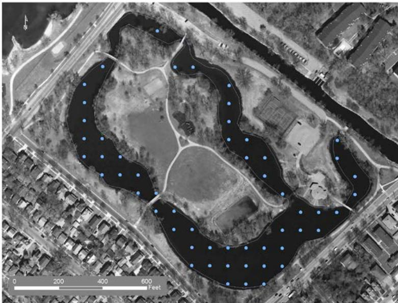
Figure 3: Point intercept sampling grid for Vilas Park Lagoon
