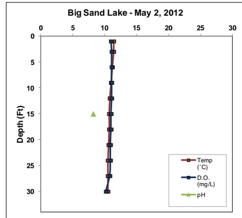
**Figure 1. Temperature, dissolved oxygen, and pH profile on Big Sand Lake.**
