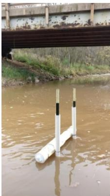
**Figure 2-2.** In situ suspended sediment sampler tube setup prior to lowering the sampler below water column. Photograph by James Blount, USGS, October 2016.
