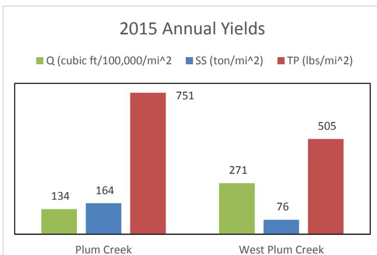
Figure 1-3. Comparison of Plum Creek and West Plum Creek annual discharge, suspended sediment, and total phosphorus yields, 2015.
