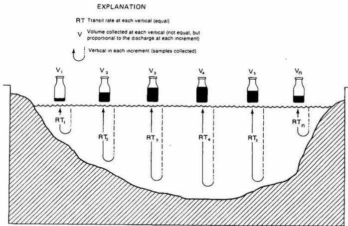
Figure 3: Example of Equal Width Increment equal transit rate (Edwards and Glysson, 1999).
