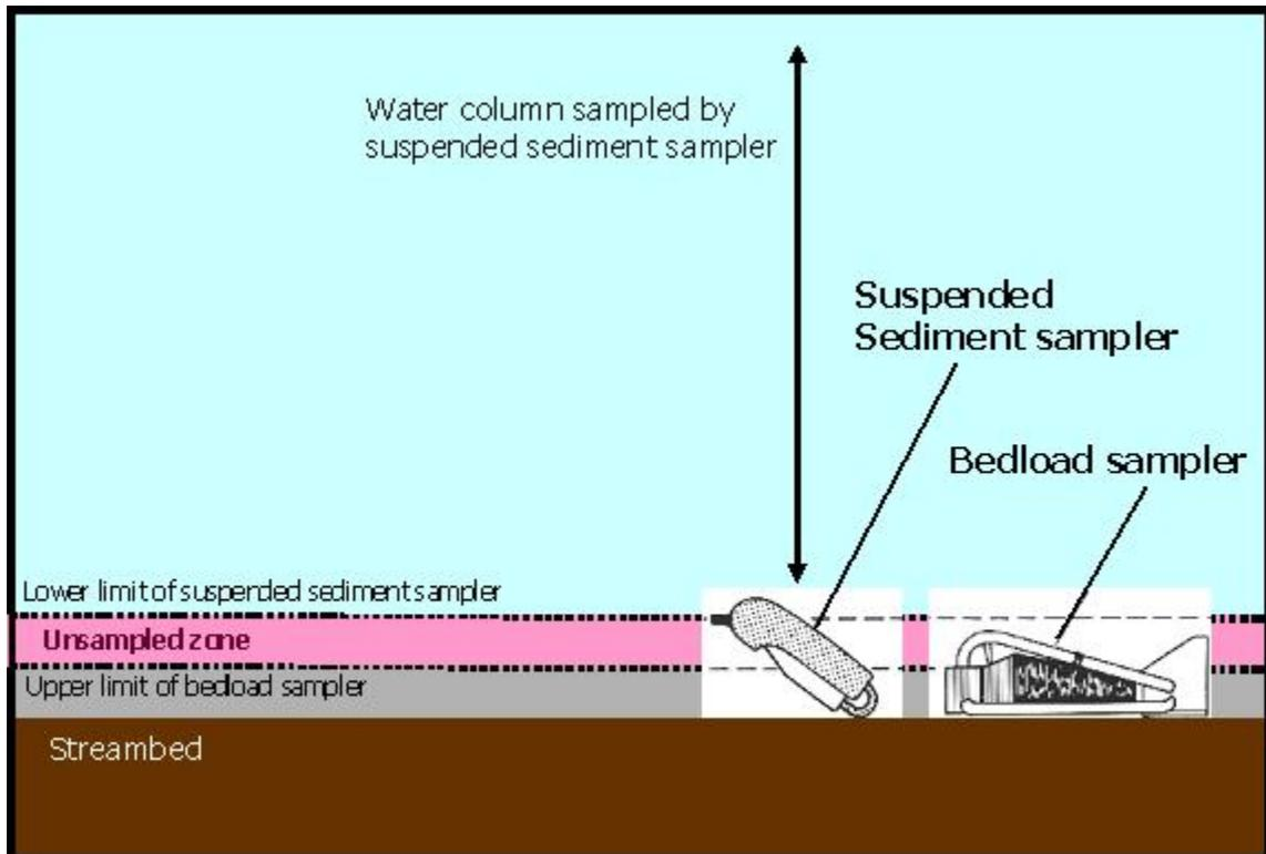
Figure 5: Diagram showing the sampling zone for suspended and bedload samplers.
