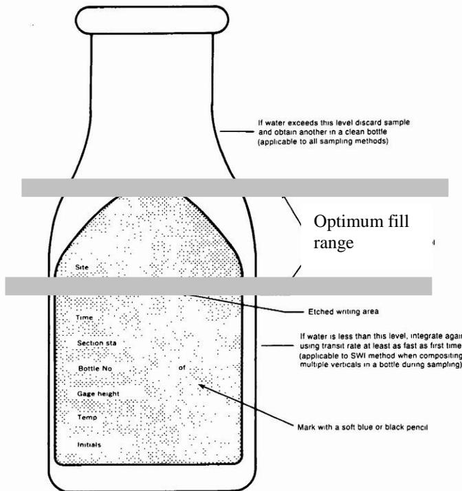
Figure 6. Example of filling of pint water bottles for suspended sediment samples (from Edwards and Glysson, 1999)
