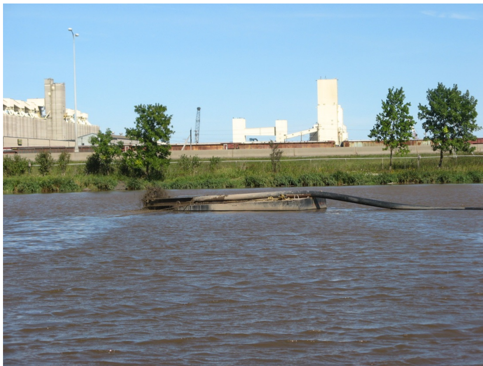
Figure 2: Surface Diffuser Used for Placement of Material
