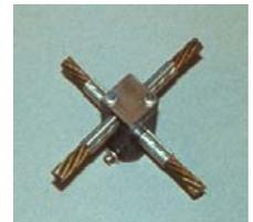
**Root Saws:** These are usually circular metal attachments with sharp metal teeth connected to cable machines that rotate to grind and cut root masses.
