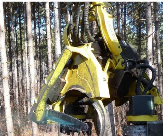
A perforated sawbar. Liquid fungicide is sprayed through small holes at the time of felling (a marker dye was added)
