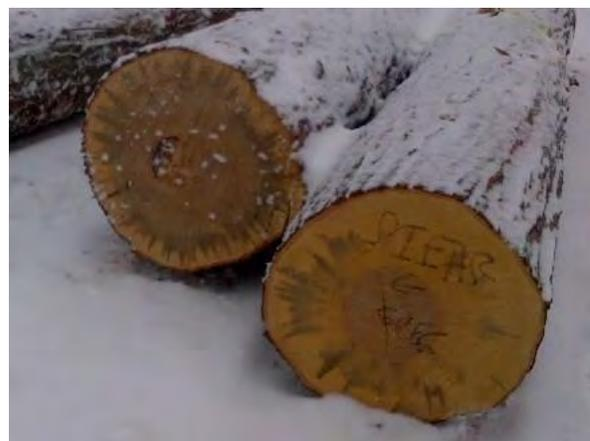
Staining in silver maple logs caused by Columbian timber beetle. Heavily stained log on left, lighter infestation on right. Photo from Algoma Lumber Co.
