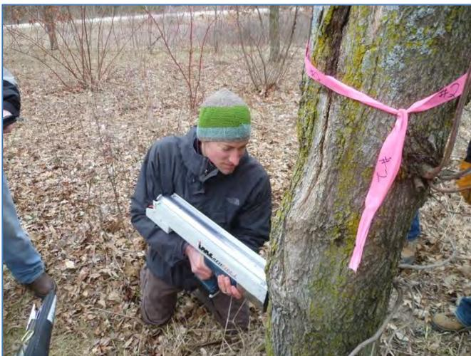
Forest health specialist, Brian Schwingle, demonstrates the high-tech resistograph drill for determining decay.
