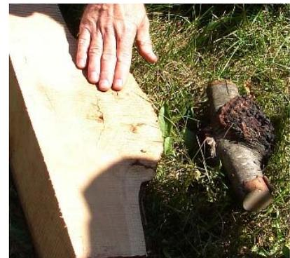
Cross section of a large black knot burl, showing sound wood with some ingrown bark.
