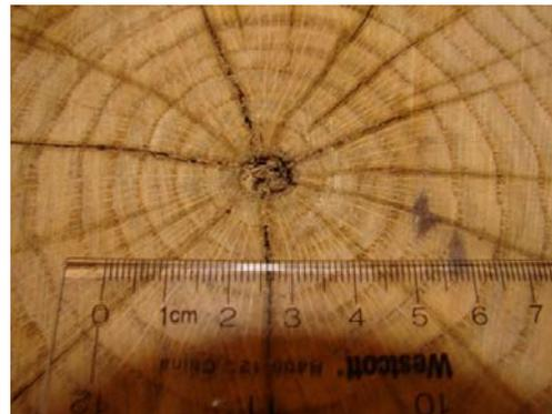
Cracks in the wood of oak running perpendicular to the annual rings, referred to as spider heart.
