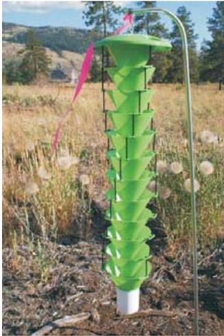
Green funnel trap can be used for EAB detection. Photo by Synergy Semiochemical.
