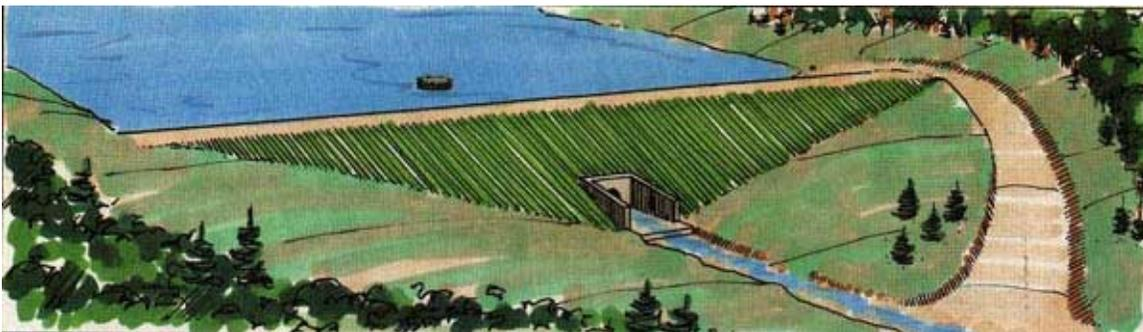
**AUXILIARY SPILLWAY (EMERGENCY SPILL- WAY)** - A secondary spillway designed to operate only during exceptionally large floods.
