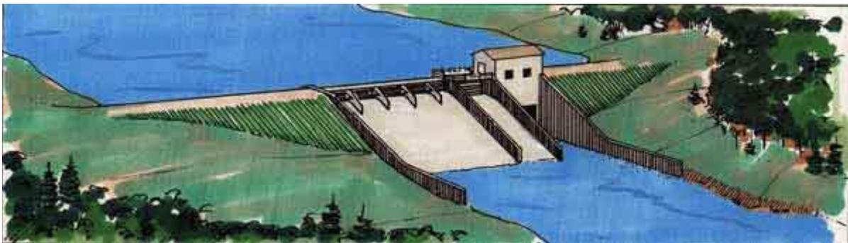
**GRAVITY DAM** - A dam constructed of concrete and/or masonry that relies on its weight for stability.
