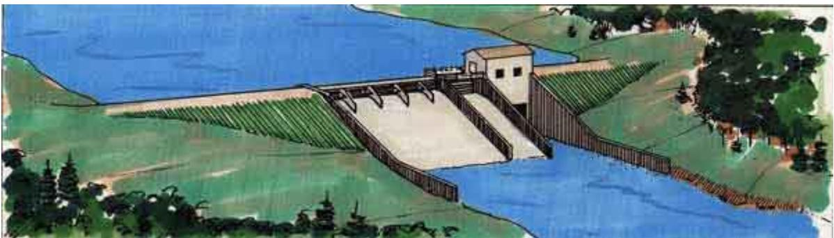
**ENERGY DISSIPATOR** - Any device constructed in a waterway to reduce or destroy the energy of fast-flowing water.
