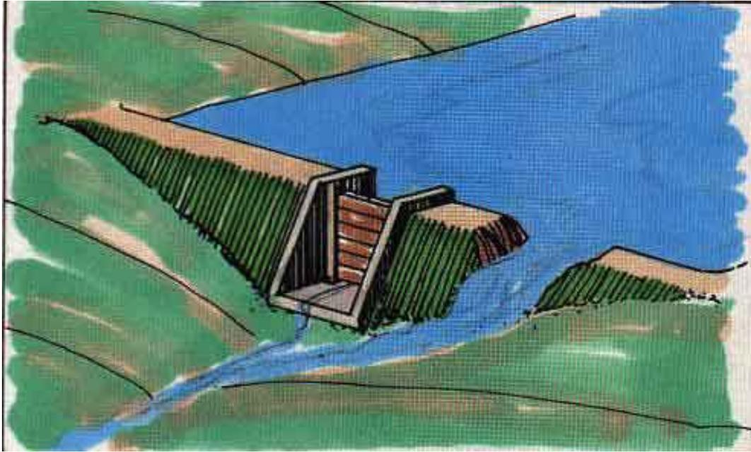
**CONDUIT** - A closed channel to convey the discharge of water through or under a dam.
