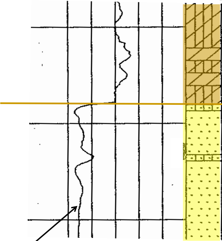
Composite ratio curve: pore pressure/ penetration rate
