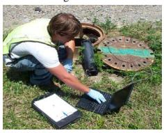
Flow meters are placed at varying locations throughout the collection system. These meters measure the amount and rate of wastewater flow in the sanitary sewer lines. The monitors are left in place for a specified period of time. Data is collected and compared to rainfall amounts over the same period. Measurements taken before and after a rainfall event indicate how much I/I contribute to the total flow of wastewater in the collection system.
