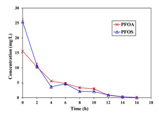
**EXHIBIT 6** The degradation of PFOA and PFOS in still bottom sample B during 16-hr electrochemical oxidation treatment
