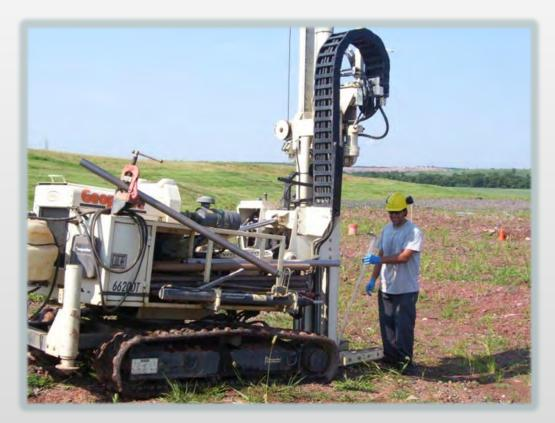
Example of direct push sampling for soil and groundwater
