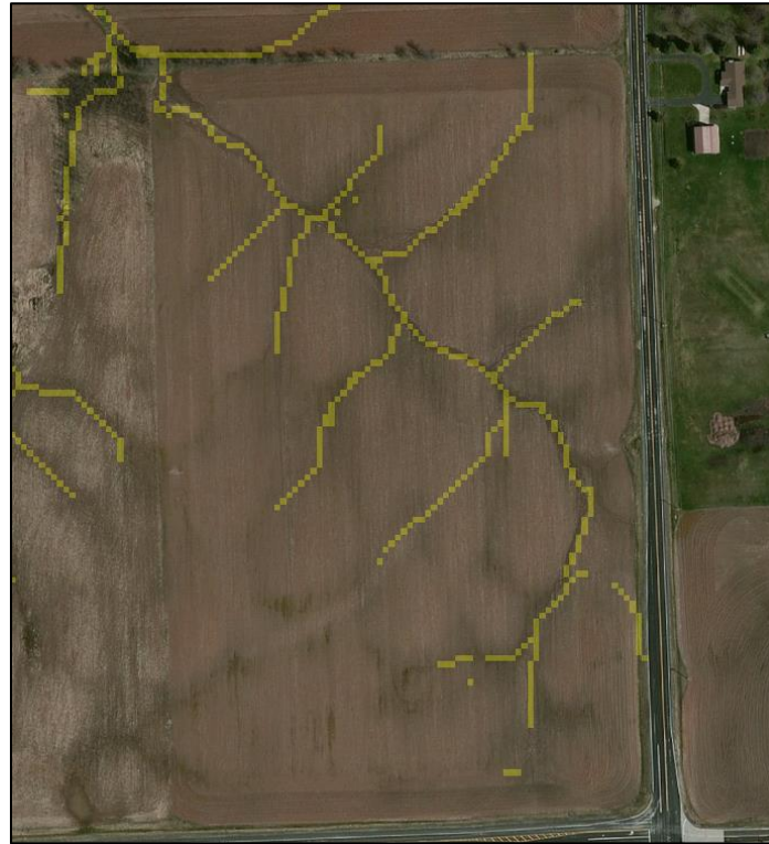
Figure 4. Yellow indicates areas of high stream power and thus potential for gully erosion. The yellow areas coincide with areas on the aerial photo that appear to be eroding.
