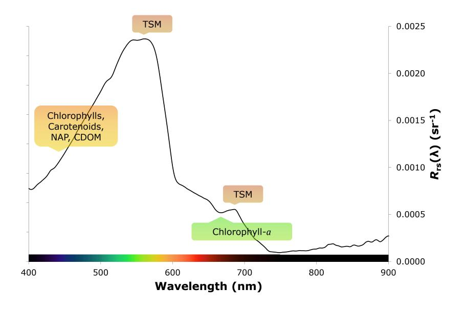
Remote sensing reflectance spectrum for Trout Lake acquired on 07/21/2015. This remote sensing reflectance spectrum is typical for many clear lakes in northern Wisconsin (NAP – non-algal particles, CDOM – colored dissolved organic matter, and TSM – total suspended matter).
