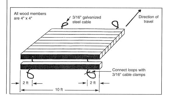
Make loops at the end of each cable for ease of transport. Secure loops with 3/16-inch cable clamps. Tuck loops under the mats during installation and use so that they don't get caught by vehicles.
