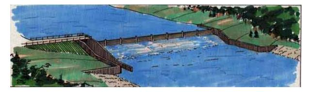
**GROIN** - That area along the contact (or intersection) of the face of a dam with the abutments.
