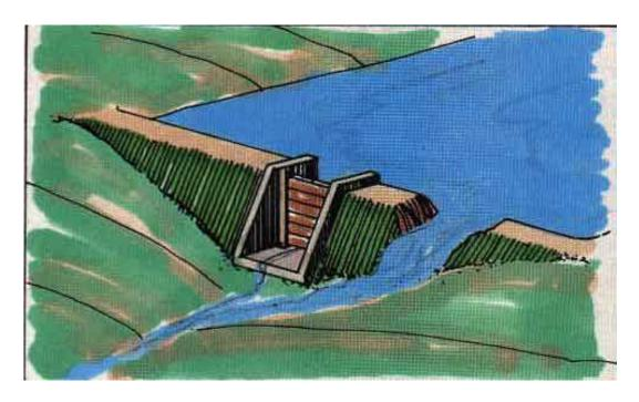
**CONDUIT** - A closed channel to convey the discharge of water through or under a dam.
