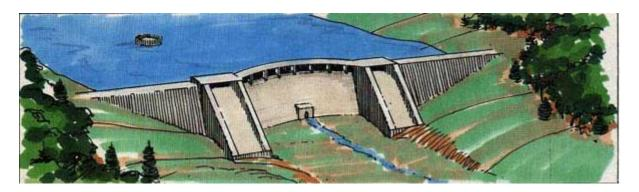
**PIPING** - The progressive development of internal erosion by seepage appearing downstream as a hole or seam discharging water that contains soil particles.
