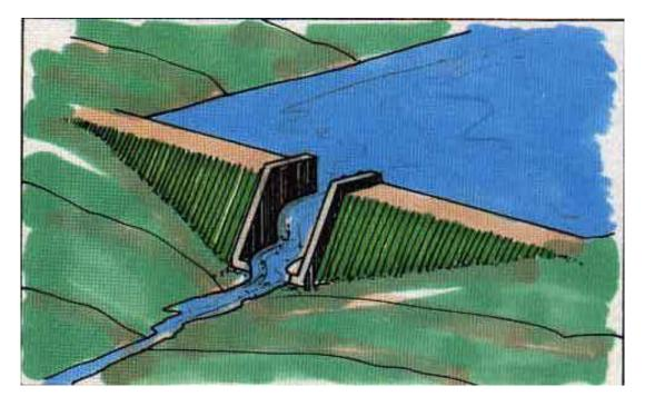
**EMBANKMENT DAM (EARTH DAM / EARTHFILL DAM)** - Any dam constructed of excavated natural materials, usually earth or rock, placed with sloping sides.
