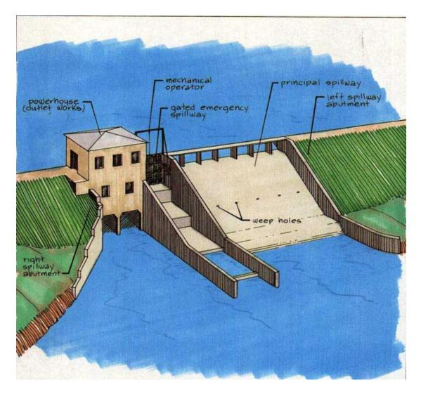
**APPURTENANT STRUCTURES** - Refers to ancillary features of a dam, such as the outlet, spillway, outlet conduit, tunnels, etc.
