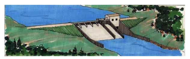
**ENERGY DISSIPATOR** - Any device constructed in a waterway to reduce or destroy the energy of fast-flowing water.
