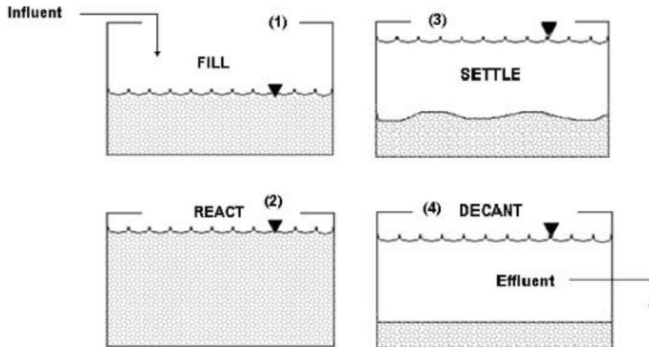
Sequencing Batch Reactor Process
