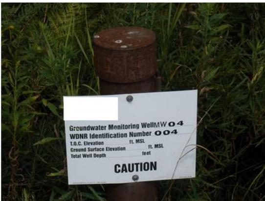
**Figure 2.** Well label attached to the well casing clearly showing the well name and DNR monitoring point ID number.
