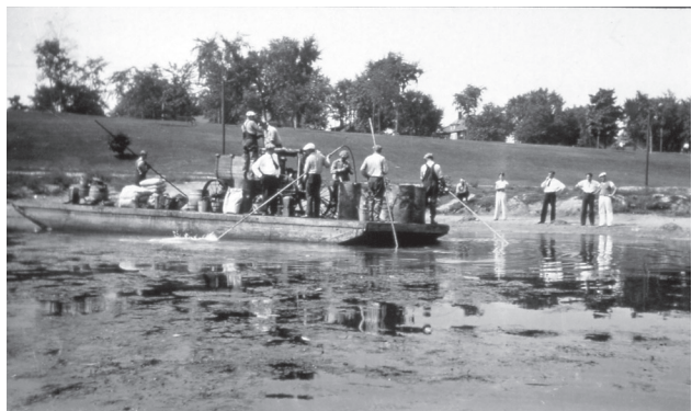
Figure 5. -Barge used in early years of copper sulfate treatments on Lake Monona. A motor boat towed the barge along the lake shoreline during spraying. (Source: Bernard Saley, originally published in Lathrop et al. 1992)
