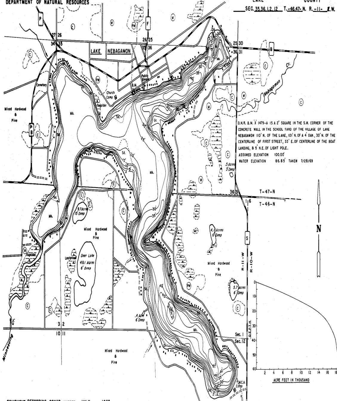
D.N.R. B.M. X 1479-A IS A 2" SQUARE IN THE S.W. CORNER OF THE CONCRETE WALL IN THE SCHOOL YARD OF THE VILLAGE OF LAKE NEBAGAMON 110' N. OF THE LAKE, 101' N. OF A 4' OAK, 30' N. OF THE CENTERLINE OF FIRST STREET, 33' E. OF CENTERLINE OF THE BOAT LANDING, 8' S. N.E. OF LIGHT POLE.
