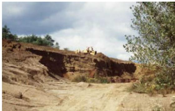
Consolidated rock may be considered stable at angles up to 90 degrees depending on several factors such as the rock type, bedding planes, zones of weakness, degree of fracturing, and resistance to erosion. For example, at one site a massive Silurian dolomite might be considered a good candidate for a vertical highwall, while that same rock at another location may not be stable in a vertical condition due to extensive fracturing, alteration or dissolution.
