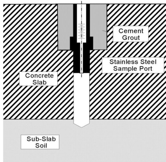
Components of the sub-slab probe: 1) small diameter hole drilled through the concrete slab 2) larger diameter hole to place and seal probe; 3) stainless steel or brass probe through which sub-slab vapor will be collected 4) sealing material such as cement grout.
