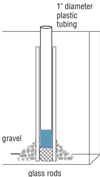
3. Place gravel so that all holes at the bottom of the 1" diameter plastic tubing are covered. The gravel will help keep sand from entering the well during pumping.
