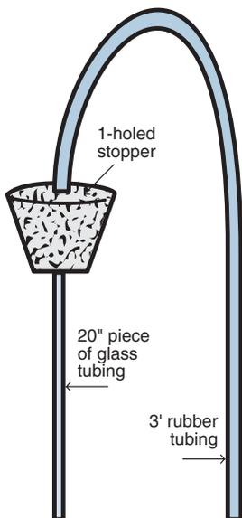
5. Attach one end of the 3' (foot) rubber tubing to glass tube extending out of the stopper.
