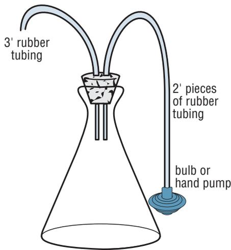
9. Insert stopper into the flask.
