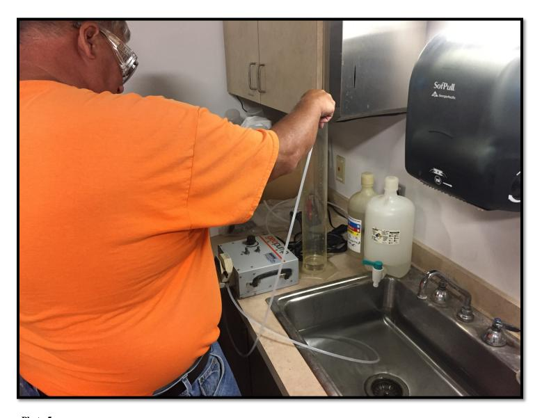
Photo 5 Description: The peristaltic pump calibration is in progress prior to dye testing pilot. Site: Tyco Fire Products
