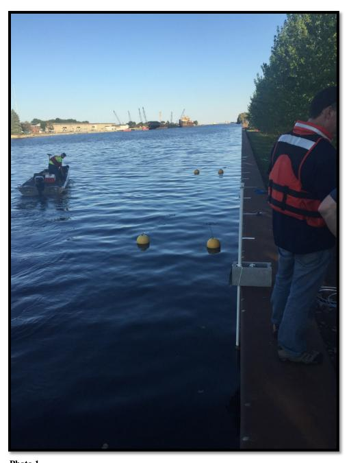
**Photo 1**Description: The CH2M SCUFA data logger set up an array in preparation for Test Number 2.
