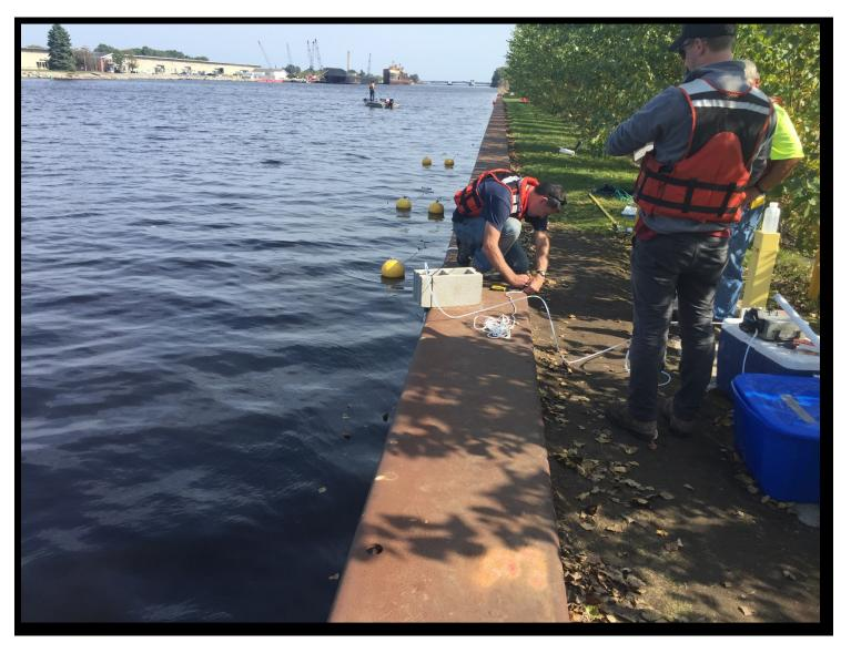
Photo 4 Description: Test Number 2's pilot dye testing injection is in progress. The SCUFA array was set up prior to commencing testing. Site: Tyco Fire Products
