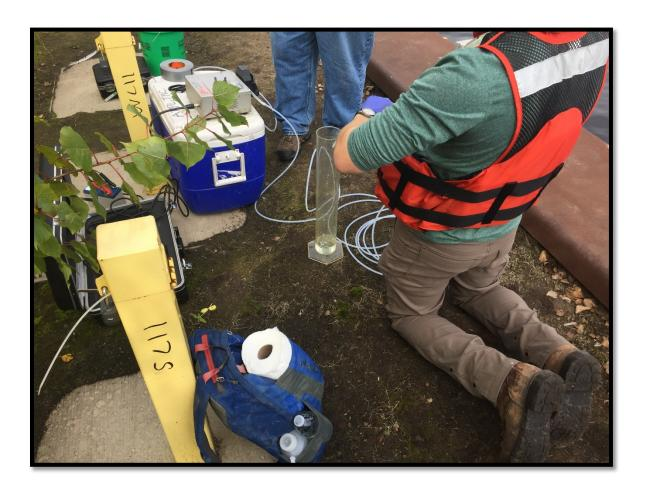
Photo 2 Description: This image displays the pilot dye testing injection point at the monitoring well MW-117M. The injection point calibration is in progress.
