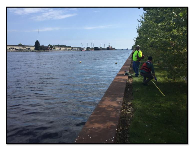
Description: The pilot dye testing is in progress for Test Number 1. The SCUFA loggers locate themselves relative to the buoy
