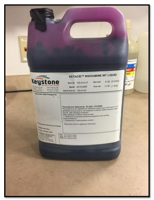
Description: Keystone KeyAcid Rhodamine WT Liquid was the dye used for the pilot tests.
