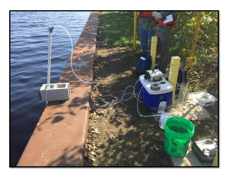
Description: This image displays the pilot dye testing injection in progress with a PVC pipe sheath used to support the injection
