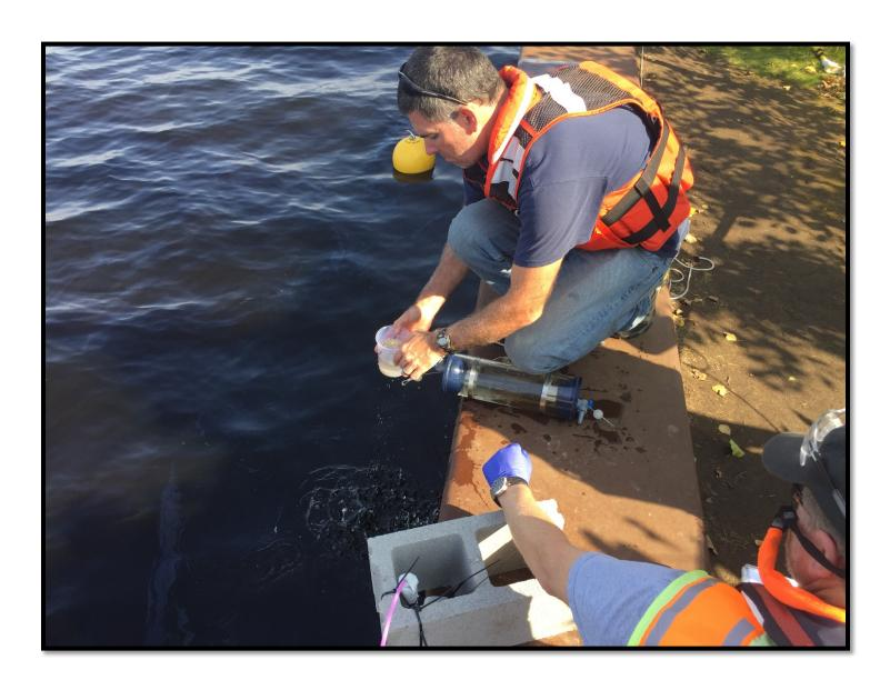
Description: The personnel are using a Van Dorn horizontal water sampler to transfer the sample for fluorescence readings. Site: Tyco Fire Products
