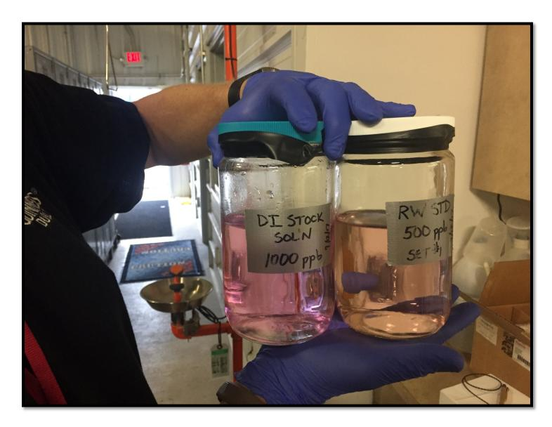
Photo 3 Description: The two glass jars indicate pilot dye testing standards for calibration. Site: Tyco Fire Products
