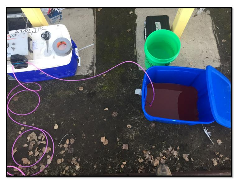
Description: This displays Test Number 2's pilot dye testing injection point at MW-1117M. The dye color appears to be a brownish-
