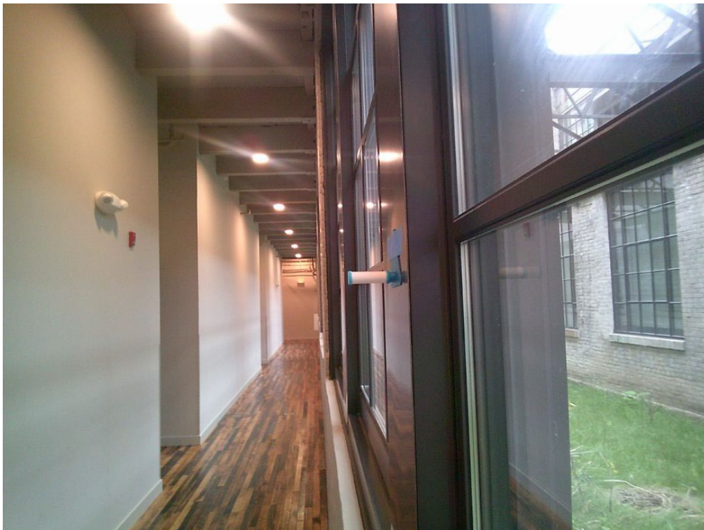
Picture 4. Passive Sampler installed in the hallway
