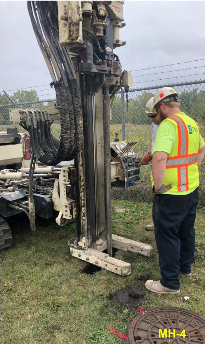
Photo 17: Geoprobe boring (MH-4-BF) within open Hydrovac borehole northeast of manhole MH-4. View to northeast; photograph taken on September 20, 2021.
