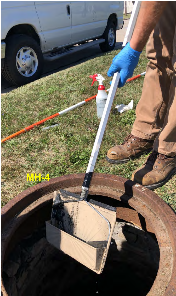
Photo 6: Sediment within manhole MH-4 being sampled with pivoted dustpan. View to northwest; photograph taken on September 1, 2021.
