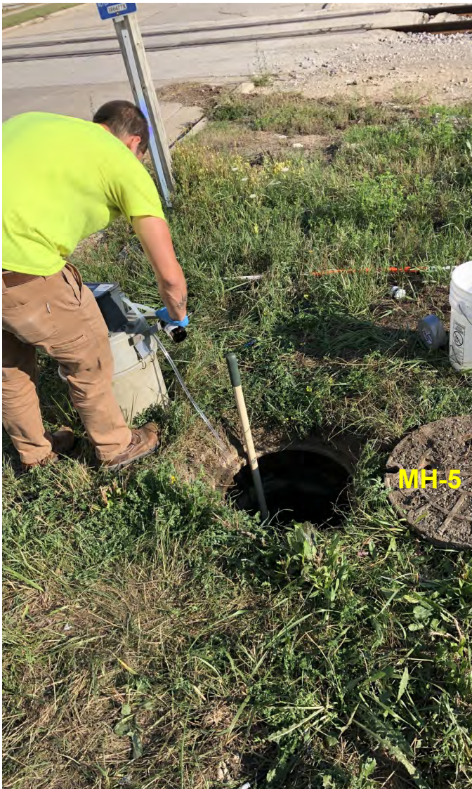
Photo 8: Water within manhole MH-5 (located in grass east of South Marina Drive) being sampled with peristaltic pump. View to northwest; photograph taken on September 2, 2021.
