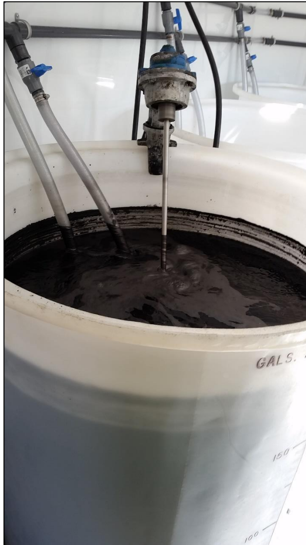
Figure 4 BAM and PFAS Degrading Bacteria batch mixing.
