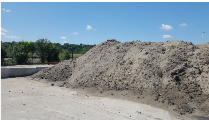
Source; Post-Dredged Dried Sediment in concrete bins
