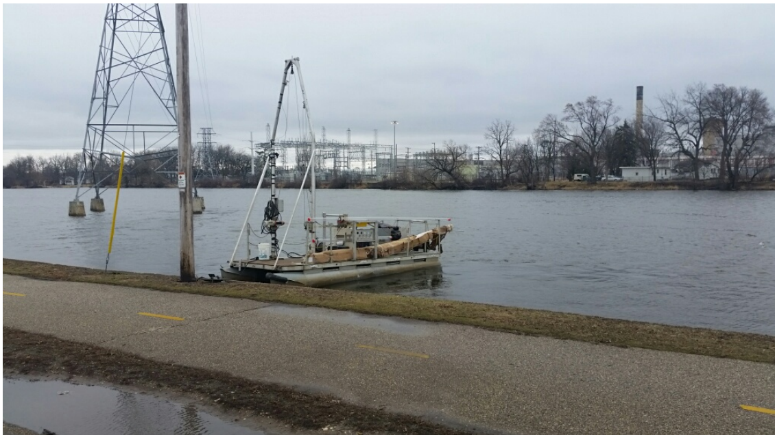
Photo 2 Coring Vessel Outfitted with A-Frame, Electric Winch, Generator, and all Necessary Sediment Coring and Collection Tools (March 9 and 10, 2016)
