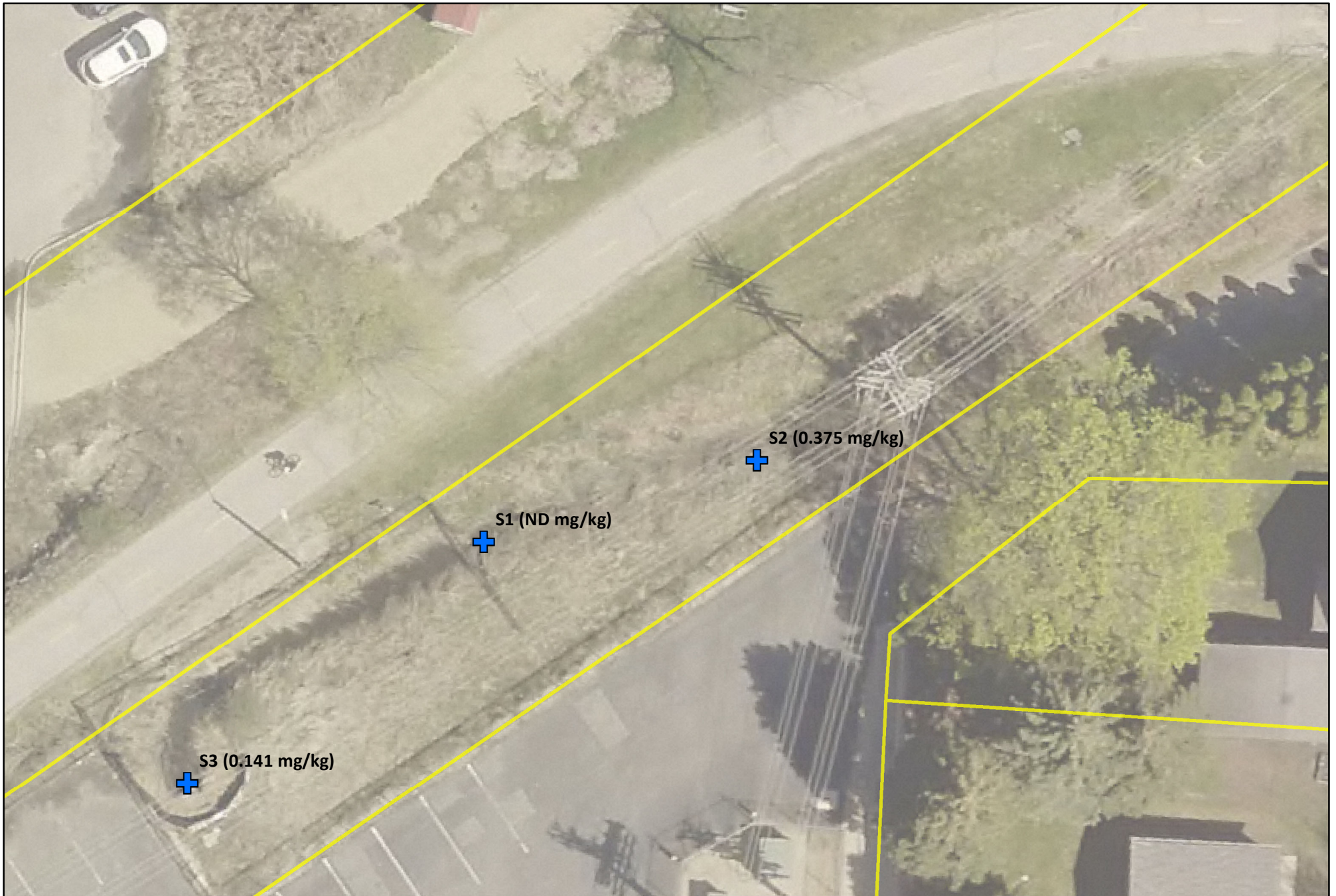
FIGURE 1 - 2018 PCB Sampling of Rain Garden Collected by City of Madison Engineering on 11/7/18. Industrial Direct Contact Residual Contaminant Level is 0.744 mg/kg.
