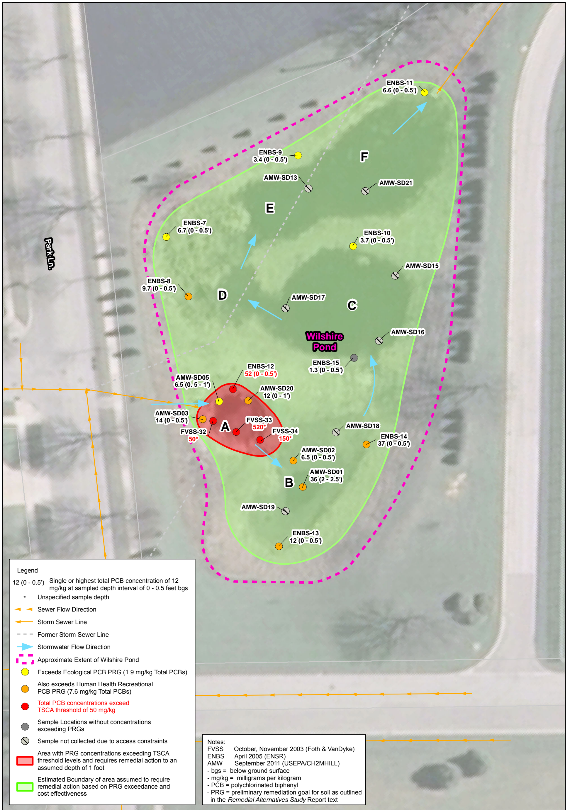
Figure 2-3 Wilshire Pond - Bank Soil and Basin Sediment PCB PRG Exceedances Feasibility Study Report Amcast Industrial Site Cedarburg, WI
