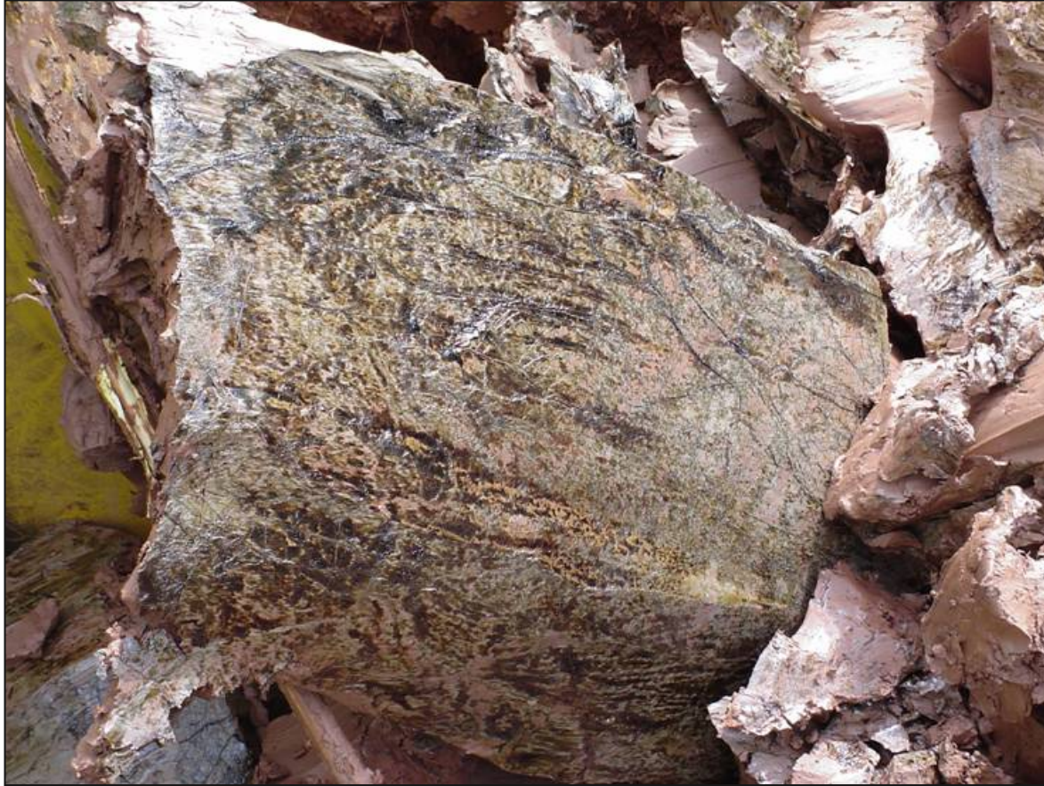
NAPL in clay fractures (cleaved from test pit sidewall)
