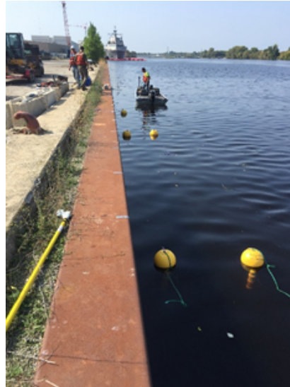
Continuously measure downstream concentrations using SCUFAs
