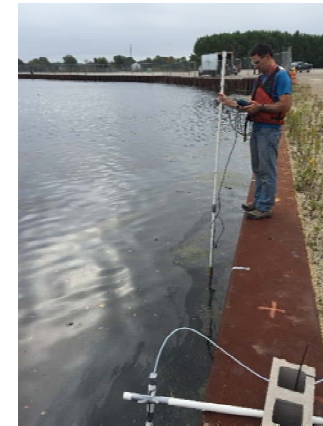
Measure stream velocities and collect surface water grab samples
