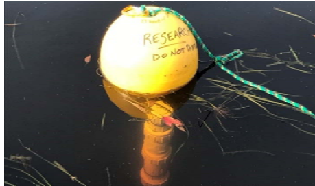
Continuously measure downstream concentrations using SCUFAs
