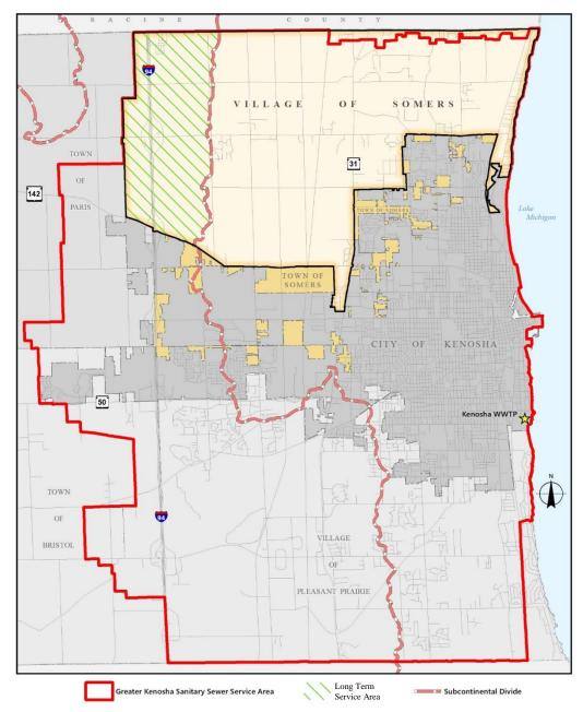
Figure 4: Greater Kenosha Sanitary Sewer Service Area
