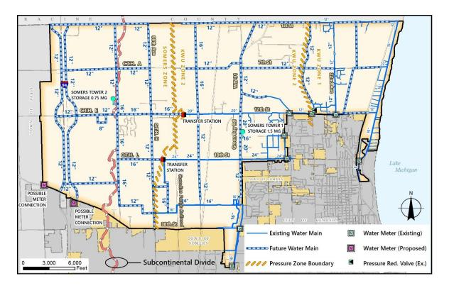
Figure 8: Concept Ultimate Water Distribution Plan
