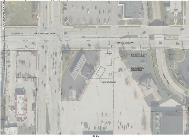
Figure 2-2. Proposed water supply pump station site plan
