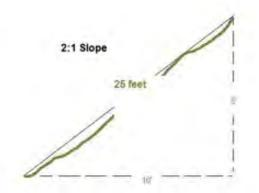
**Figure 1:** Example measurement of bank slope height. In this example, the bank slope height is 25 ft or the length of the hypotenuse (Source: NRCS Erosion Calculator).
