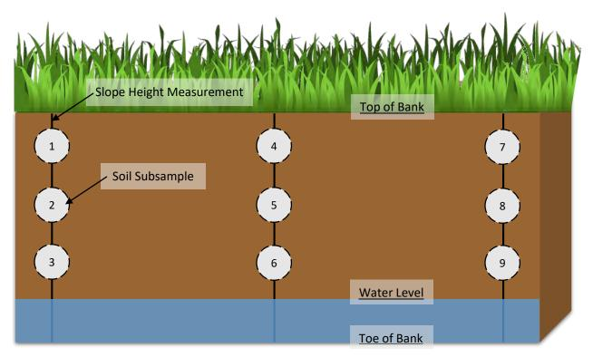
Figure 2: Diagram of soil sampling locations for a typical eroding bank
