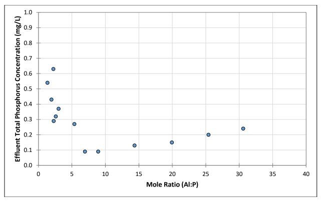
Figure 2-3: Brodhead WWTF chemical phosphorus removal pilot testing results (spring 2016)
